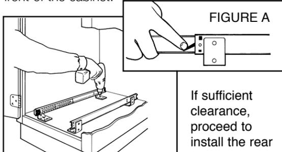
If sufficient clearance, proceed to install the rear 2 screws and refer to enclosed RV Series Door Mount Instruction Sheet for door mounting.
