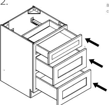
8-2. Slide your completed drawer into the cabinet until the glides click into place securing the drawer.
