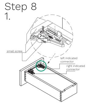
8-1. Locate the right and left glide connectors. Place them on the under side of the drawer (triggers inward) and secure them to the drawer front, side, and floor using four small screws per connector.
