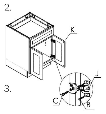
9-2. Locate the pre-drilled dimple on the inside lip of the face frame. Then drill a 3/4" deep pilot hole with a 3/32 drill bit.
