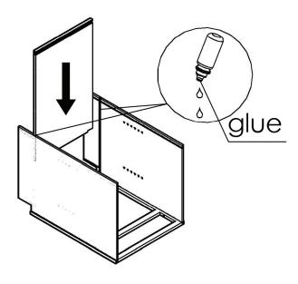
2. Slide the floor board into the parallel grooves on the walls. Make sure the floor board notch fits into the grooves on the face frame. Make sure the groove on (the) floor board is inward toward the inside of the cabinet.
