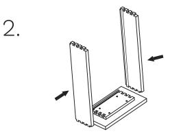
7-2. Using a rubber mallet lightly pound each drawer side into place. Line up the teeth and the grooves on the drawer front to the teeth and grooves on each side (grooves inward).
