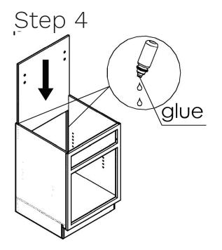
4. Flip the cabinet upright and slide the back wall into the parallel grooves on the back side of the cabinet (finished side inward).Be sure to slide it into the grooves on the floor board.
