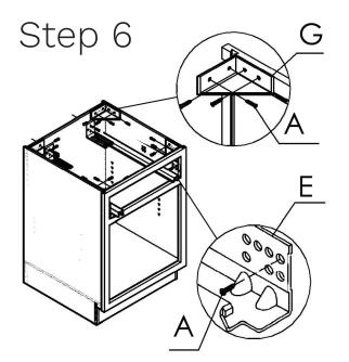
6. Flip the cabinet onto the back side (face up). Place one corner bracket into each corner on the inside of the cabinet. This will secure the face frame and back wall to the left and right sides of the cabinet.
