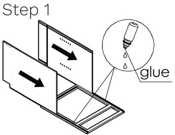
1. Place the face frame face down. Place a bead of glue in the dovetail groove. Slide the left and right sides into the vertical grooves (holes inward). Wipe away any excess glue.
