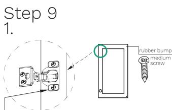
9-1. Place the door face down and set each hinge into place. Line up the corresponding screw holes on the door with the corresponding holes on the hinge. Secure the hinges to the door with two medium screws per hinge. Place one rubber bumper on the inside of each corner (opposite of the hinges).
