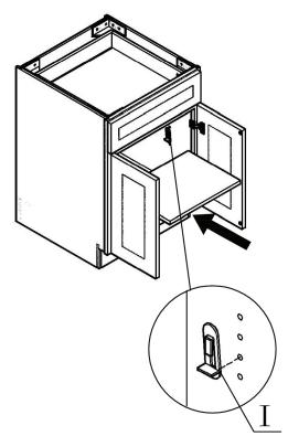
10. Place your shelf clips in the holes on the side walls of your cabinet (lip side down). Place the shelf on to the clips and lightly press down until the shelf clicks into place.
