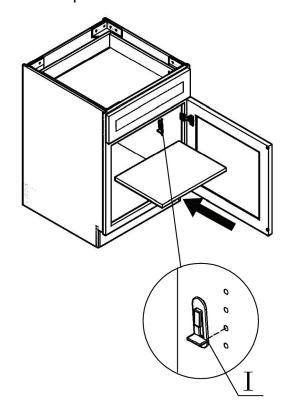
10. Place your shelf clips in the holes on the side walls of your cabinet (lip side down). Place the shelf on to the clips and lightly press down until the shelf clicks into place.
