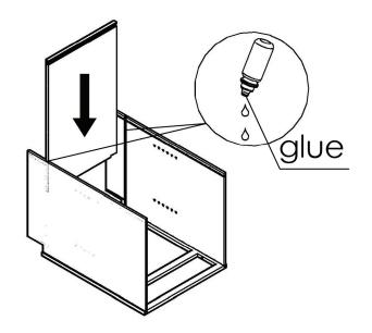
2. Slide the floor board into the parallel grooves on the walls. Make sure the floor board notch fits into the grooves on the face frame. Make sure the groove on (the) floor board is inward toward the inside of the cabinet.
