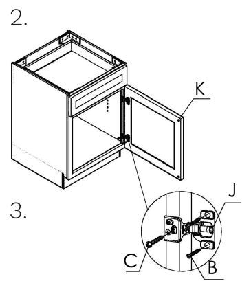
9-2. Locate the pre-drilled dimple on the inside lip of the face frame. Then drill a 3/4" deep pilot hole with a 3/32 drill bit.
