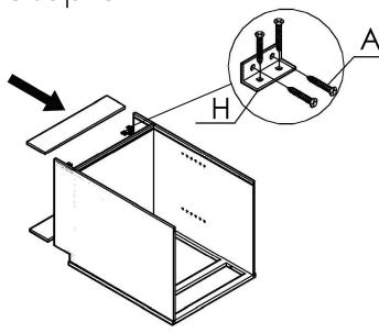
3. Place the small toe kick into the grooves below the floor board on the back side of the cabinet (opposite of face) paint side out.
