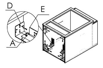
5. Locate L brackets. Match the holes on the brackets to the corresponding holes on the inside of the back wall. Use small screws to attach them to the cabinet.
