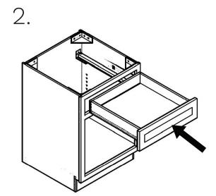
8-2. Slide your completed drawer into the cabinet until the glides click into place securing the drawer.
