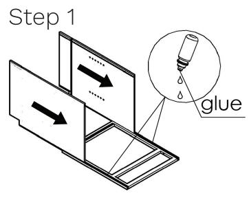
1. Place the face frame face down. Place a bead of glue in the dovetail groove. Slide the left and right sides into the vertical grooves (holes inward). Wipe away any excess glue.
