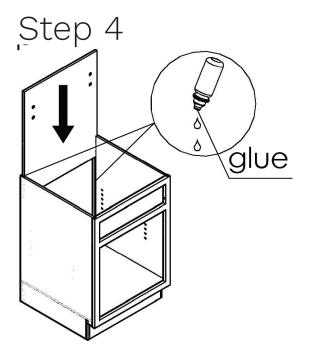
4. Flip the cabinet upright and slide the back wall into the parallel grooves on the back side of the cabinet (finished side inward). Be sure to slide it into the grooves on the floor board.
