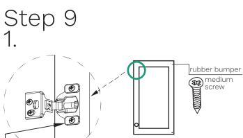
9-1. Place the door face down and set each hinge into place.
