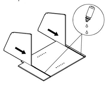
1. Locate the side wall without the lip and start with the side wall paint side down. Apply wood glue to the dovetail grooves. Slide the top and bottom of the cabinet into the parallel grooves (paint side out).
